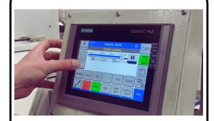
Open the channel manually on the bar feeder
