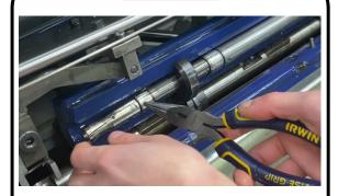
You just locate the pin. And press with the pliers
